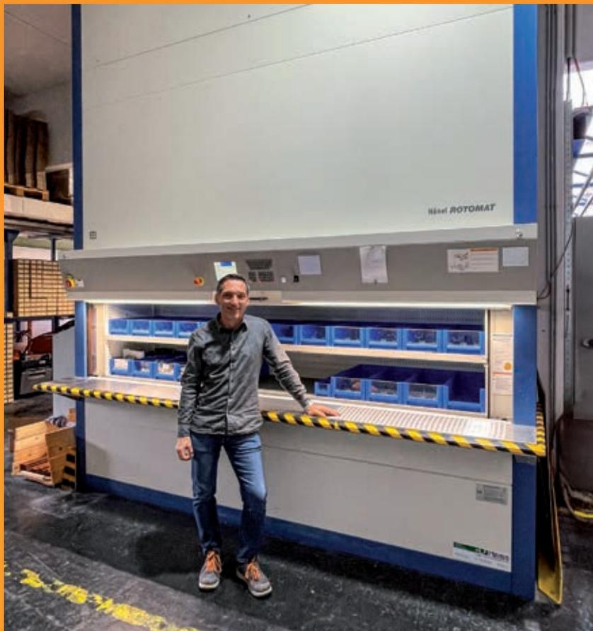
The new carousel, which is affectionately known internally as a paternoster, offers a remarkable 48m<sup>2</sup> of storage space on a 15 m<sup>2</sup> footprint. Around 800 spare parts - naturally provided with master data and article numbers - find their allocated space and enable smooth maintenance and repairs of our special machines. "This further important digitalisation step now ensures smooth maintenance processes," says a delighted Gernot Baumgartner, our Head of Production.
