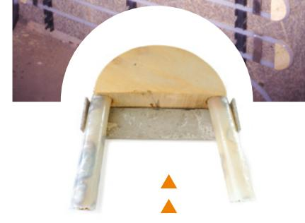
The first bending model for the first system walls was affixed to the pipe on the wall and plastered over
